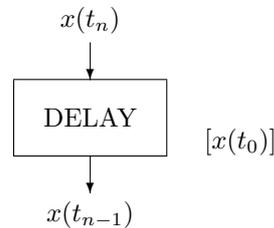
The DELAY block delays its input by one step. The optional parameter  $x(t_0)$  is used as initial value. If not declared,  $x(t_0)$  defaults to zero. The DELAY block can be found in the *Mathematics – Loops* category.
