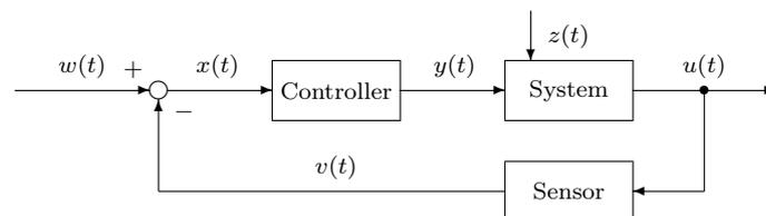
The task of a control cycle is to keep a controlled process variable  $u$  within in a narrow range close to a given set point  $w$ . The variable  $u$  usually depends on  $w$  and a disturbance variable  $z$ .
